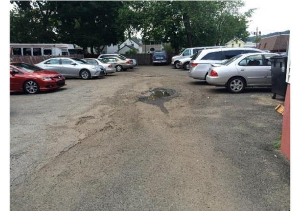
Parking spaces can be replaced with pervious pavement to capture and infiltrate stormwater. Two rain gardens can also be built in front of the church to capture, treat, and infiltrate runoff from the roof. A preliminary soil assessment suggests that more soil testing would be required before determining the soil's suitability for green infrastructure.
