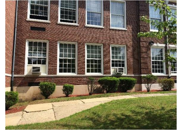
A rain garden can be built in front of the school to capture, treat, and infiltrate runoff from the roof by disconnecting and redirecting the downspouts nearby. A preliminary soil assessment suggests that more soil testing would be required before determining the soil's suitability for green infrastructure.
